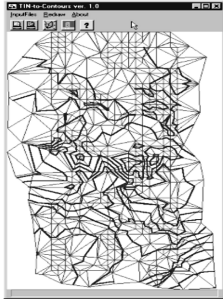
Fig. 8.40 The generated contours of 4m interval using photogrammetrically datasets (Drumbuie, Kyle of Lochash, north-west Scotland)
